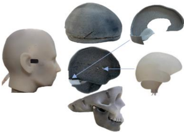
Figure 4: Skin, top skull, arachnoid trabeculae, falx-tentorium, bottom skull, jaw, and brain surrogates of the current version of Instrumented Human Head Surrogate (IHHS 5.0) developed by the DII Department of the University of Padua.
