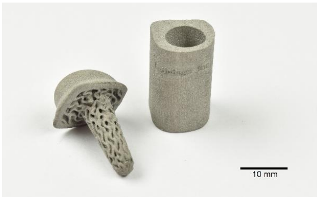
Figure 3: Sintered finger implant (left) and sinter support (right)
