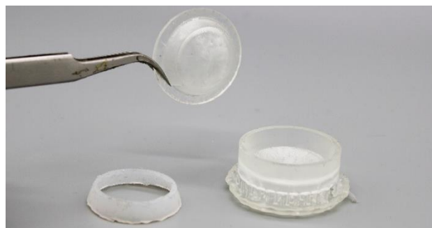
Figure 12: 3D printed molds for silicone casting gasket.
