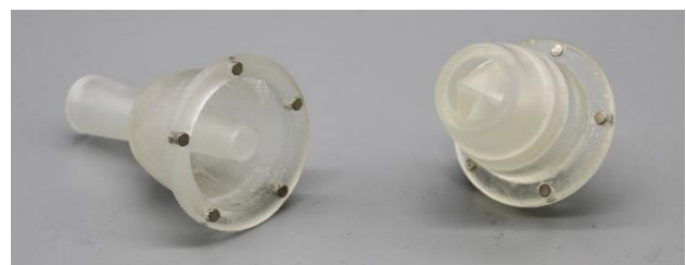
Figure 8: Initial breakaway chest drain valve concept; Left is the male part with hollow protrusion. Right includes housing and cross slit valve.
