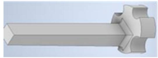
Figure 3: Positioner. The plunger like object holds the RNI in place above the RW opening between its round recesses and the inner membrane inlay wall.
