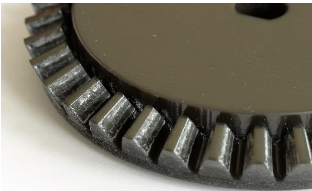
Figure 2: The contact pattern on the gear in drive direction shows an evenly distributed wearout along the upper half of the teeth.
