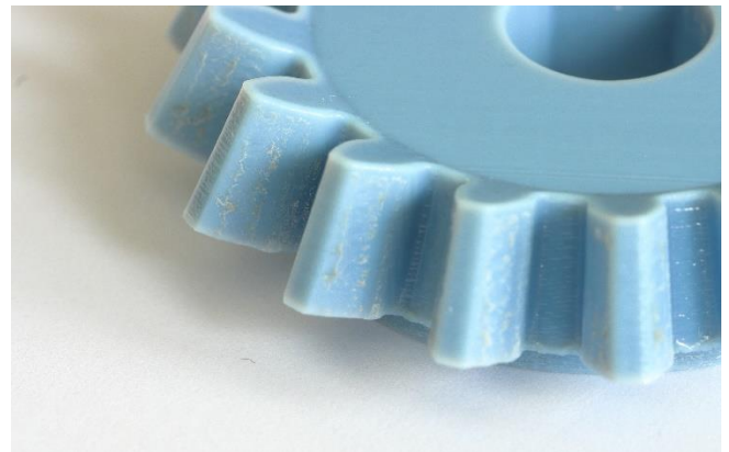
Figure 4: Wearout marks on the pinion in drive direction show only light rub-on of material from the gear, but no signs of abrasion.
