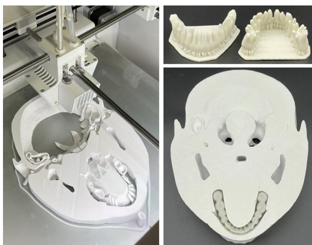
Figure 3: Additive Manufacturing of the head and neck phantom components, during FDM printing (left), teeth with support structure (top right), segment of the oral cavity with teeth (bottom right).
